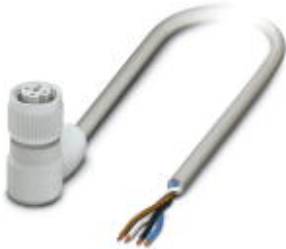
Sensor/Actuator cable, 4-position, PP-EPDM halogen-free, Gray RAL 7035, Free cable end, on Socket angled M12, A-coded, with 3 LEDs, Cable length: 10 m, Hygienic design, with plastic knurl
