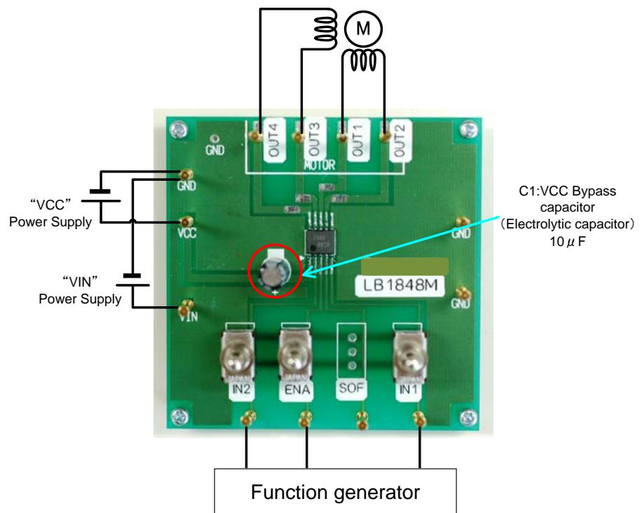
(Circuit diagram of the evaluation board)
