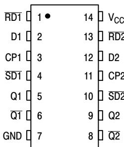
Figure 2. PIN ASSIGNMENT
