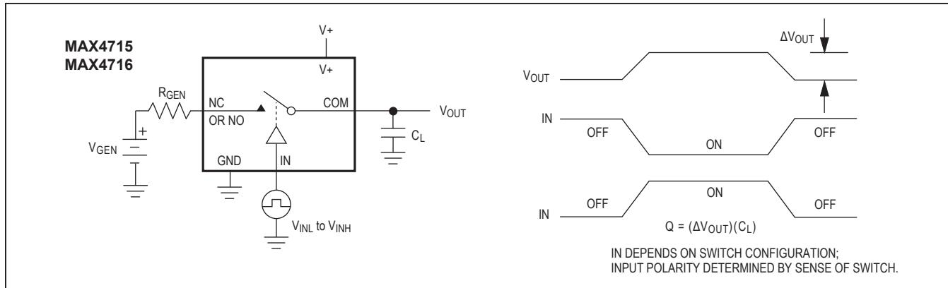
Figure 2. Charge Injection
