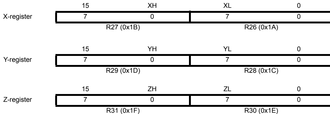
Figure 4-3. The X-, Y-, and Z-registers
