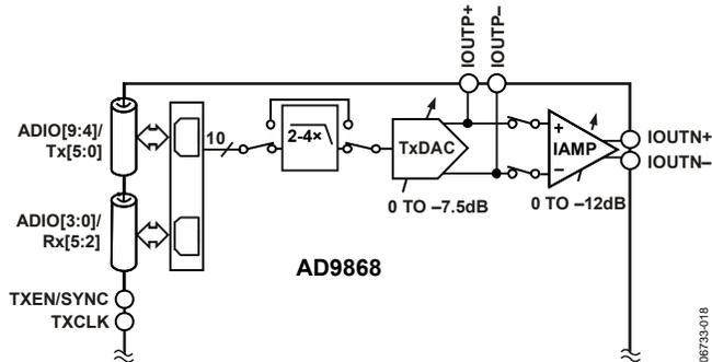
Figure 18. Functional Block Diagram of Tx Path
