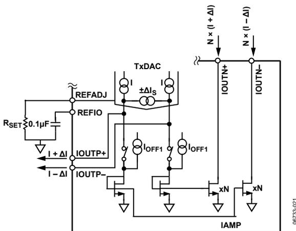
Figure 21. Equivalent Schematic of TxDAC and IAMP
