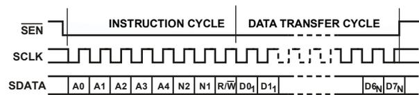
Figure 4. SPI Timing, LSB First
