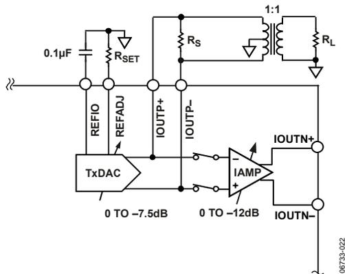
Figure 22. TxDAC Output Directly via Center-Tap Transformer
