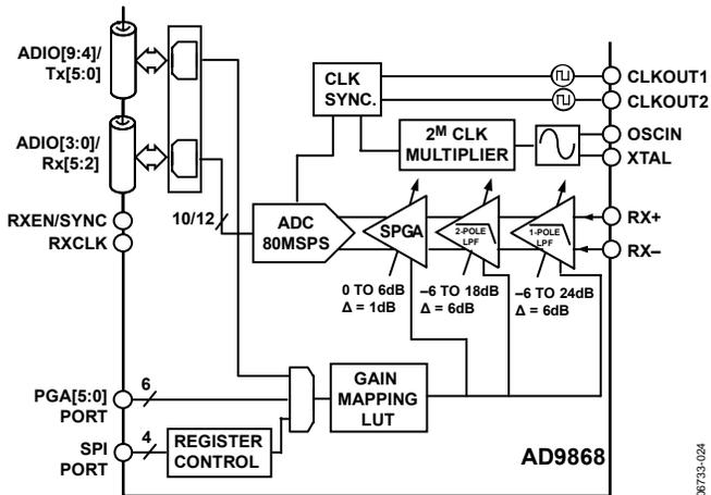
Figure 24. Functional Block Diagram of Rx Path
