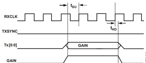
Figure 16. Updating RxPGA via Tx[5:0] in Full-Duplex Mode
