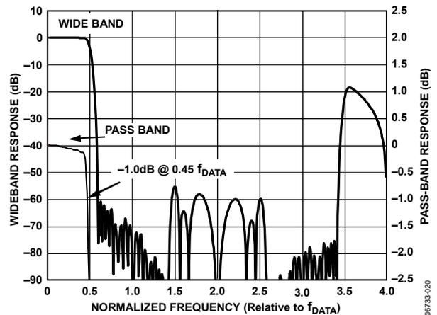
Figure 20. Frequency Response of 4× Interpolation Filter (Normalized to  $f_{DATA}$ )
