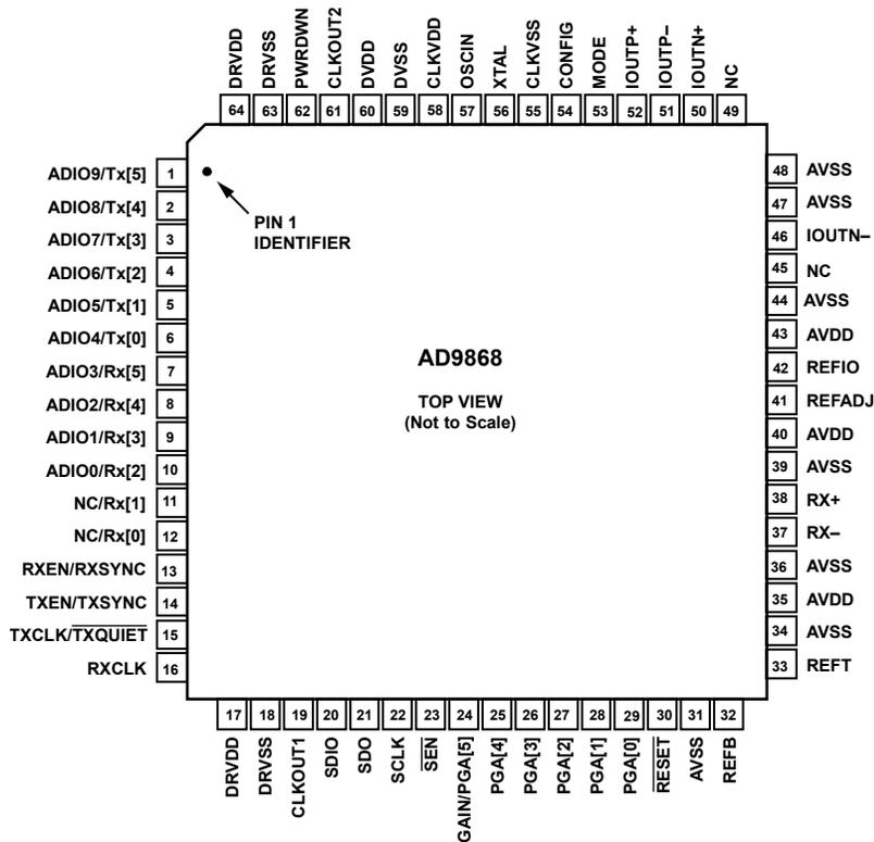
Figure 2. Pin Configuration
