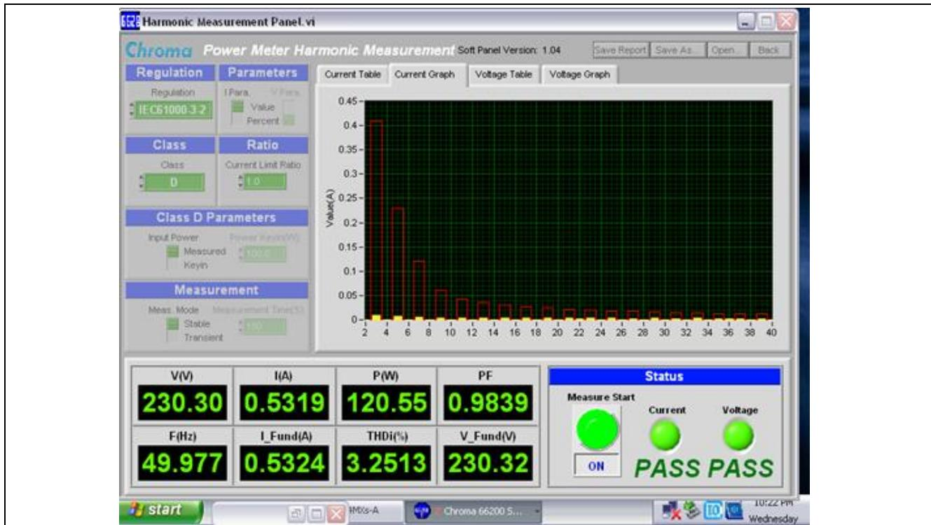
Figure 16 Input Current Harmonic Spectrum at Full Load and  $V_{IN} = 230$  VAC
