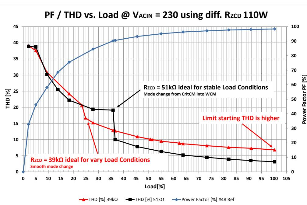
Figure 11 PF and THD versus Load
