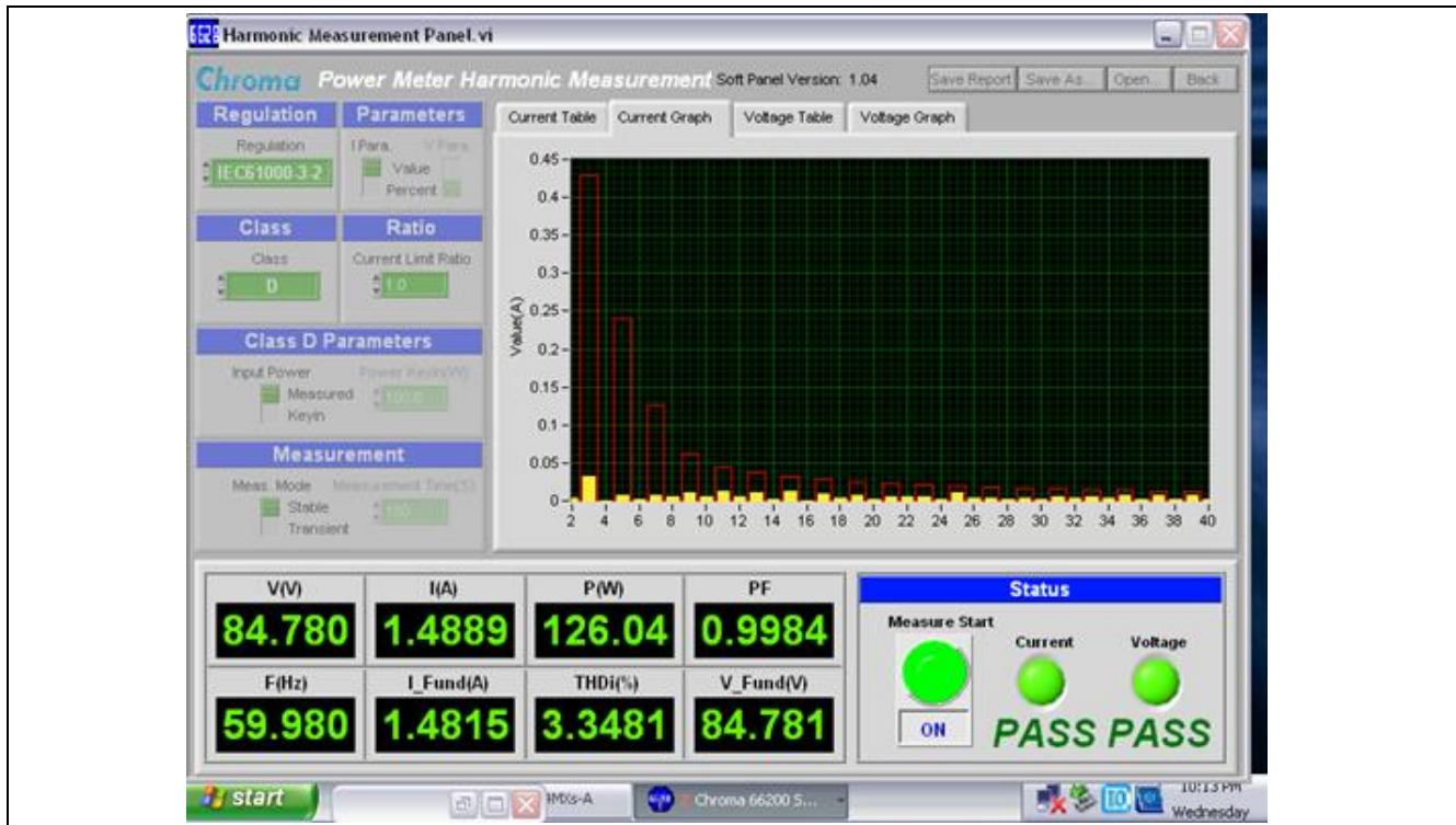
Figure 15 Input Current Harmonic Spectrum at Full Load and  $V_{IN} = 85$  VAC
