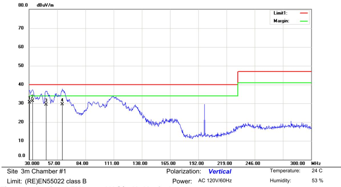
**Figure 27 Radiated EMI -- 120VAC/60Hz Vertical**
