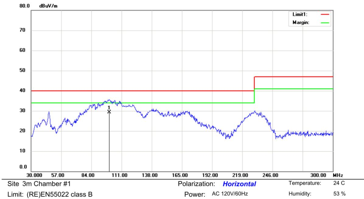
**Figure 26 Radiated EMI -- 120VAC/60Hz Horizontal**
