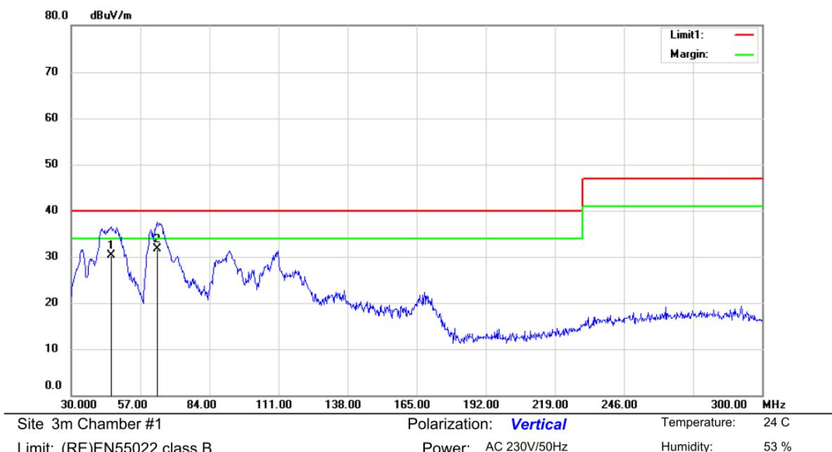
**Figure 25 Radiated EMI -- 230VAC/50Hz Vertical**
