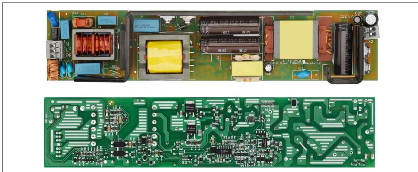
Figure 1 Demonstration Board of 110 W / 54 V LED Driver
