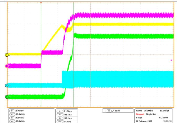
Figure 5: AC Input Voltage 85V<sub>ACIN</sub>, Full Load
