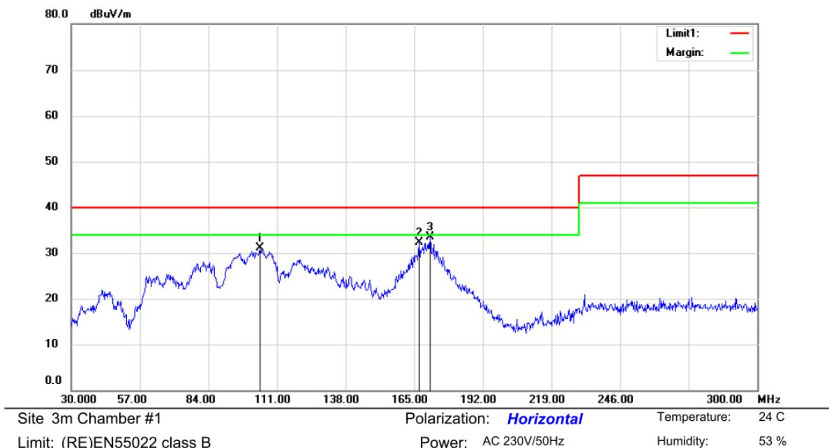
**Figure 24 Radiated EMI -- 230VAC/50Hz Horizontal**
