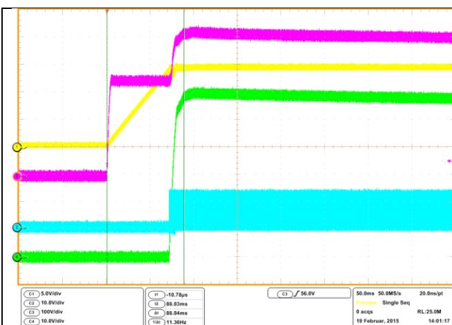
Figure 6: AC Input Voltage 230V<sub>ACIN</sub>, NO Load
