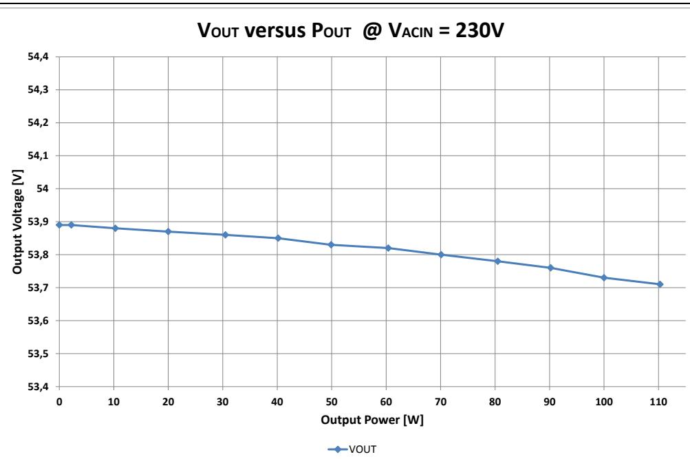
Figure 10 Output Voltage  $V_{OUT}$  versus  $P_{OUT}$
