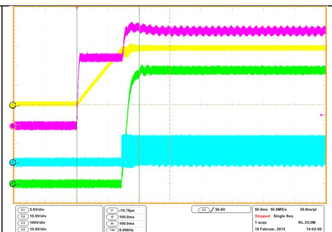
Figure 7: AC Input Voltage 230V<sub>ACIN</sub>, Full Load
