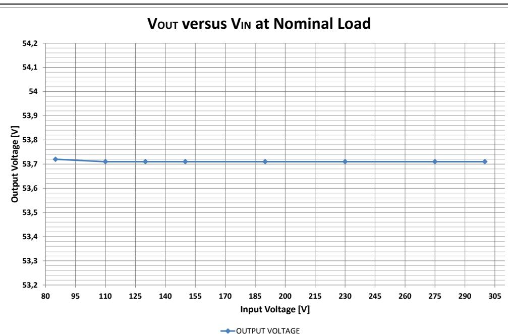
Figure 3 DC Output Voltage at Different  $V_{IN}$  Values
