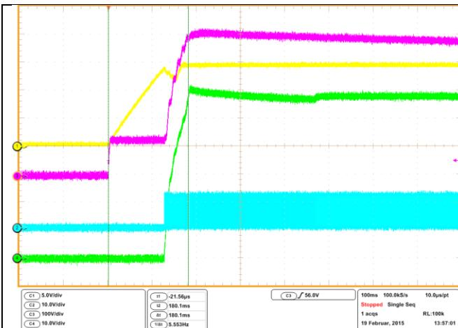
Figure 4: AC Input Voltage 85V<sub>ACIN</sub>, NO Load
