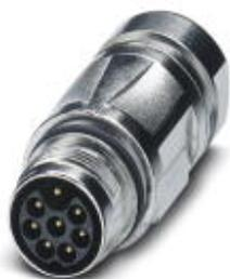
Coupler connector, straight, SPEEDCON locking, M17, Number of positions: 7+PE, Type of contact: Male connector, Crimp connection, shielded: yes, Cable diameter: 10 mm...12.5 mm
