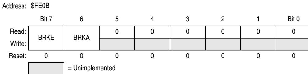
**Figure 19-4. Break Status and Control Register (BRKSCR)**
