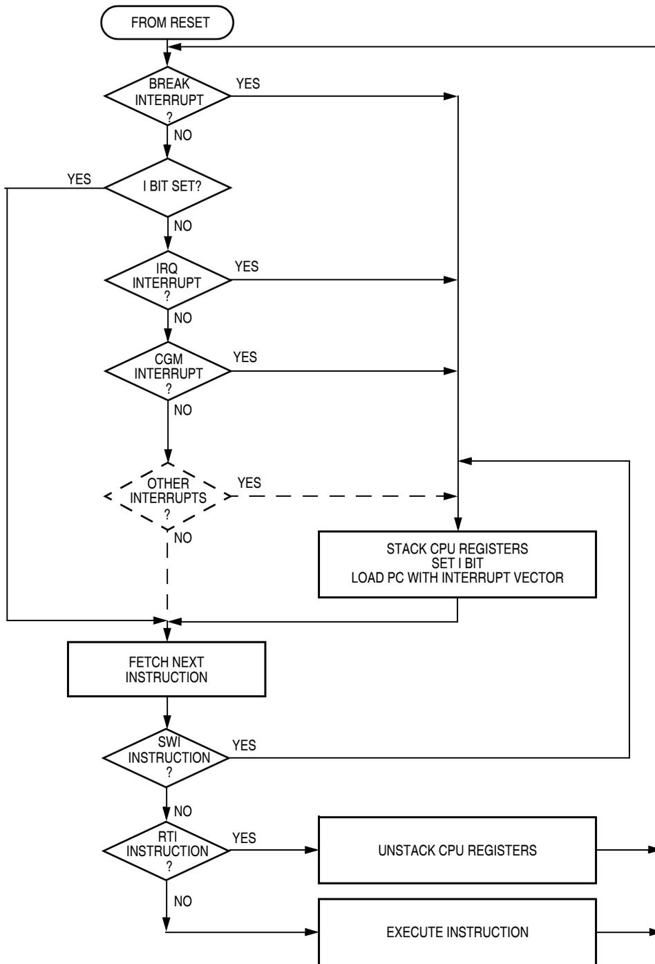
Figure 14-10. Interrupt Processing
