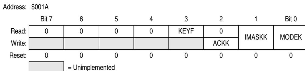
**Figure 9-4. Keyboard Status and Control Register (INTKBSCR)**
