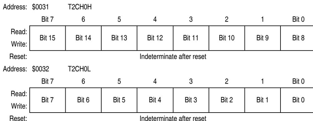
**Figure 18-10. TIM2 Channel Registers (T2CH0H/L:T2CH5H/L) (Sheet 1 of 3)**
