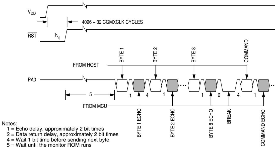
**Figure 19-17. Monitor Mode Entry Timing**
