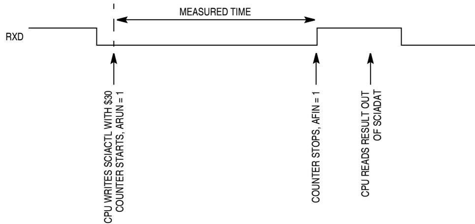
**Figure 13-22. Bit Time Measurement with ACLK = 1, Scenario A**
