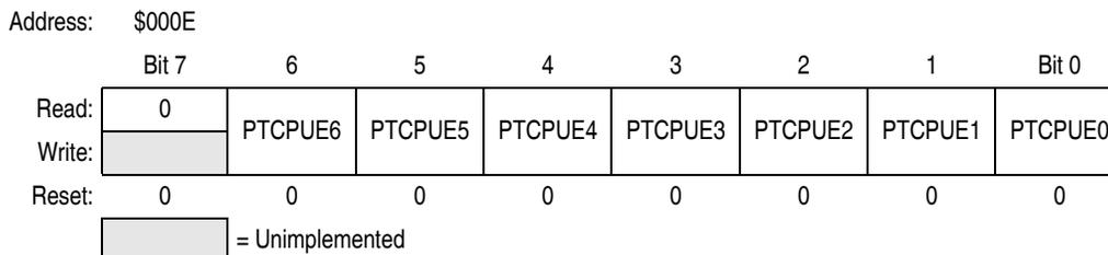
**Figure 12-12. Port C Input Pullup Enable Register (PTCPUE)**
