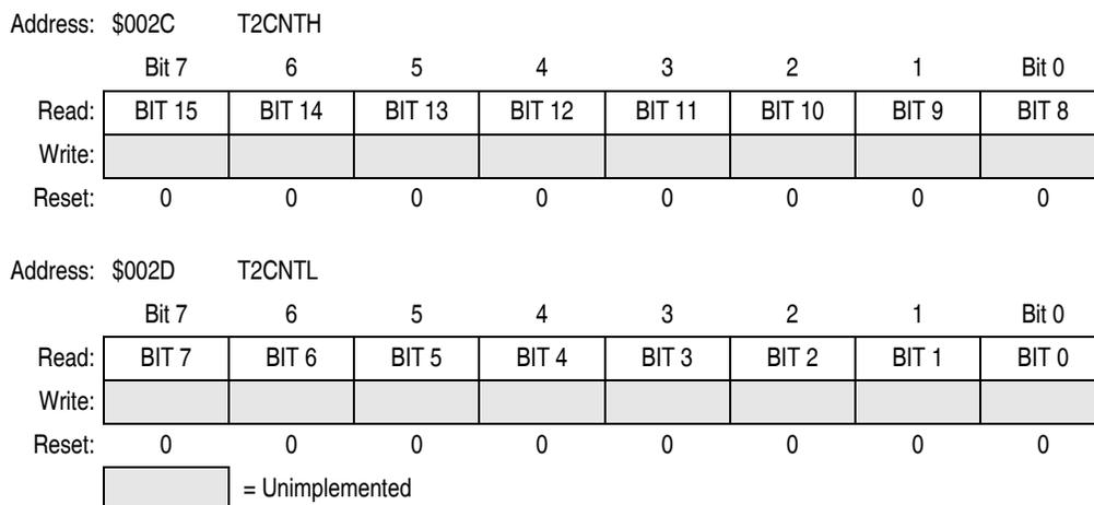
**Figure 18-6. TIM2 Counter Registers (T2CNTH and T2CNTL)**
