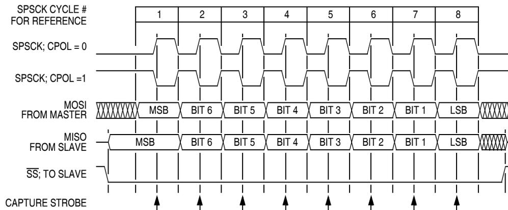
**Figure 15-5. Transmission Format ( $CPHA = 0$ )**
