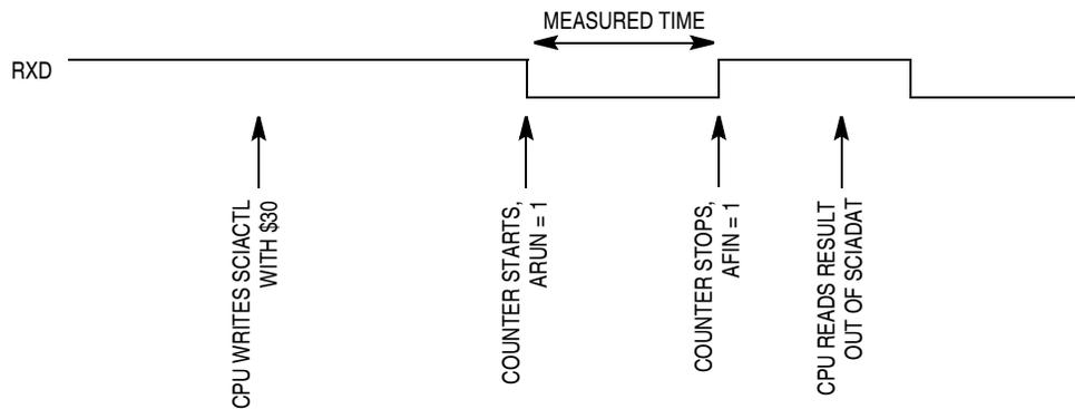
**Figure 13-23. Bit Time Measurement with ACLK = 1, Scenario B**
