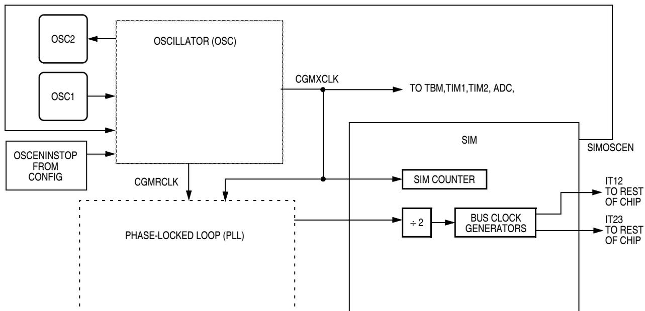
**Figure 14-3. System Clock Signals**
