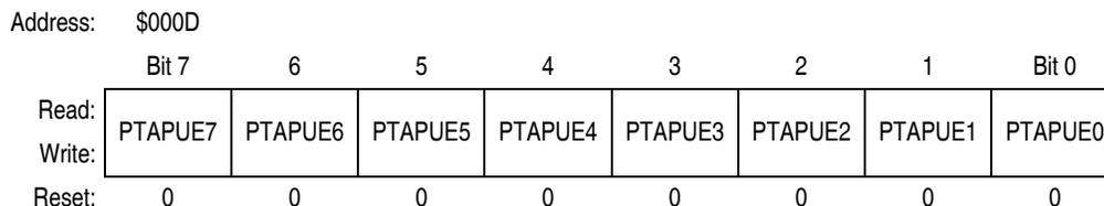
**Figure 12-5. Port A Input Pullup Enable Register (PTAPUE)**
