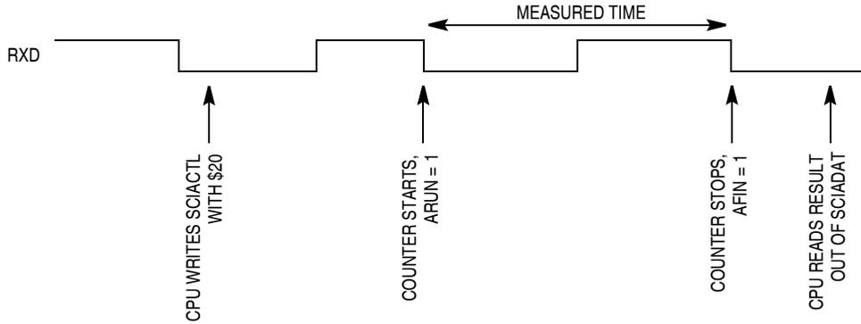
**Figure 13-21. Bit Time Measurement with ACLK = 0**
