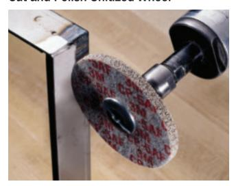
Cut and Polish Unitized Wheels are long lasting and aggressive for heavy duty blending and finishing with uniform results. The layered "unitized" construction of this wheel provides an excellent starting point for jobs requiring the availability of small diameters and narrow widths.
