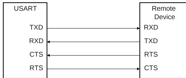
Figure 20-15. Connection with a Remote Device for Hardware Handshaking
