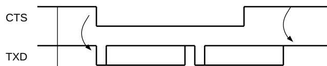
Figure 20-17. Transmitter Behavior when Operating with Hardware Handshaking
