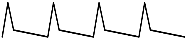
FIGURE 11. VOLTAGE ACROSS R WITHOUT RC
