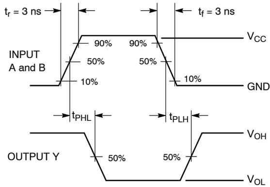
Figure 3. Switching Waveforms
