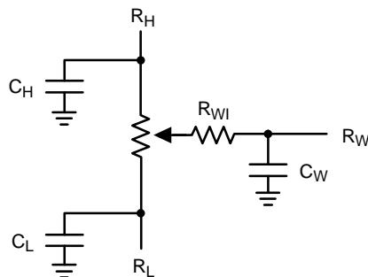
**Figure 4. Potentiometer Equivalent Circuit****Table 3. ABSOLUTE MAXIMUM RATINGS**
