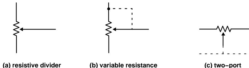
Figure 6. Potentiometer Configuration
