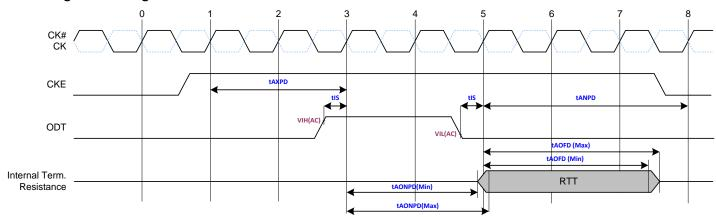
Note: Both ODT to Power Down Endtry and Exit Latencies tANPD and tAXPD are not met, therefore Power-Down Mode timings have to be applied.
