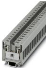
Feed-through terminal block, Connection method: Screw connection, Cross section: 0.2 mm 2 - 4 mm 2 , AWG 24 - 12, Width: 6.2 mm, Color: gray, Mounting type: NS 15
