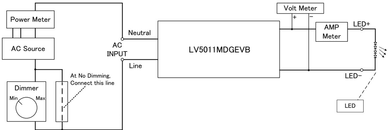
**Figure1.** LV5011MDGEVB Recommended Test Set Up
