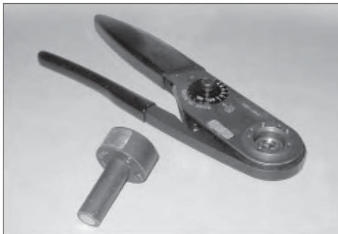
Crimp tooling M317 and locator VGE1 0077A
