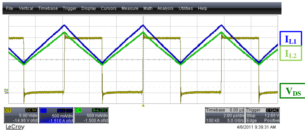
Figure 4. Operational Waveforms, V_{IN} = 12\text{ V} , R_{OUT} = 6\ \Omega
