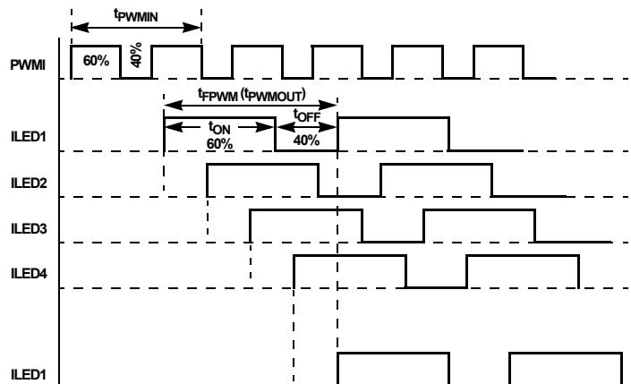
**FIGURE 25. ISL97692 4 -CHANNELS PHASE SHIFT TIMING ILLUSTRATION**
