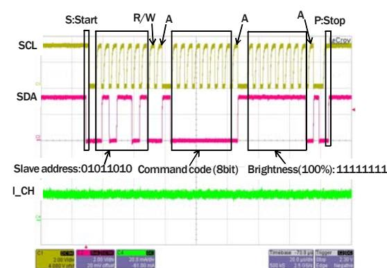
**FIGURE 18.  $I^2C$  CONTROL TIMING AND CHANNEL CURRENT (100% DIMMING, ISL97694A)**
