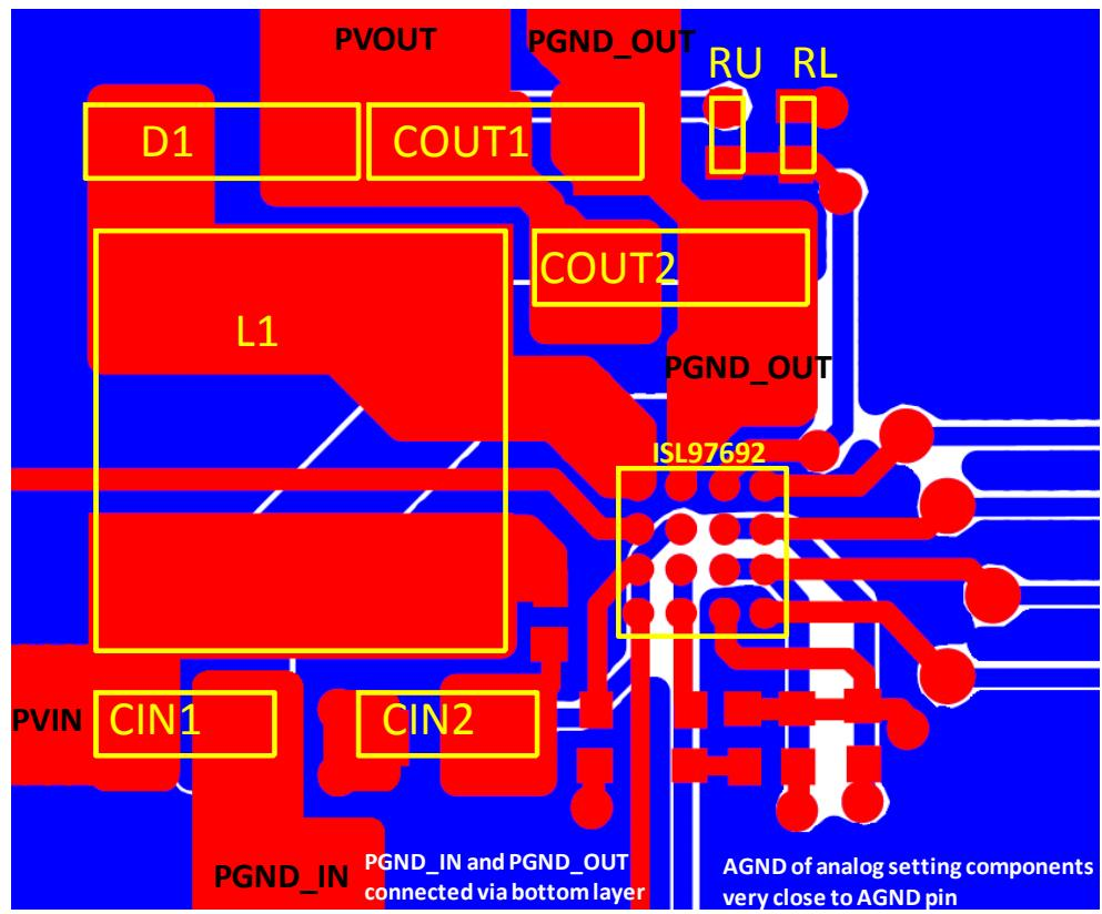
FIGURE 34. EXAMPLE OF PCB LAYOUT of ISL97692 WLCSP
