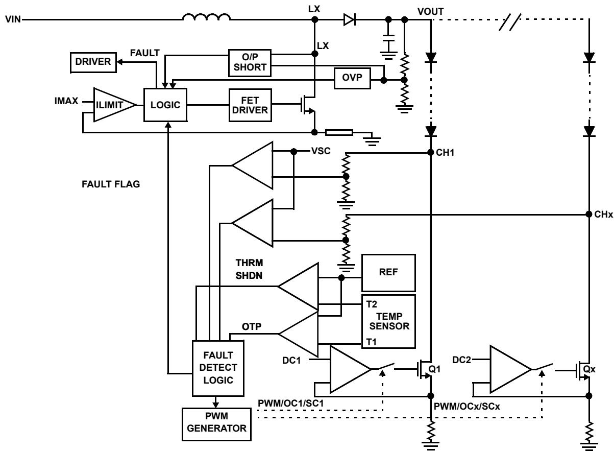
FIGURE 35. ISL97692, ISL97693, ISL97694A SIMPLIFIED FAULT PROTECTIONS
