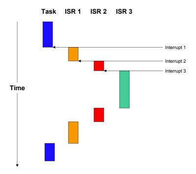
For applications requiring short interrupt latency, you may re-enable interrupts inside an ISR by using <code>OS\_EnterNestableInterrupt()</code> and <code>OS\_LeaveNestableInterrupt()</code> within the interrupt handler.
