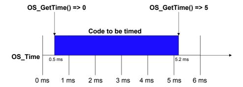
The call to  $OS_Timing_Start()$  calculates the starting value at 5,000 cycles, while the call to  $OS_Timing_End()$  calculates the ending value at 52,000 cycles (both values are kept track of internally). The measured execution time of the code in this example would therefore be (52,000 - 5,000) = 47,000 cycles, which corresponds to 4.7 ms.
