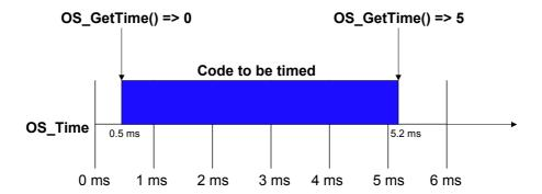
For many applications, low-resolution measurement may be fully sufficient for your needs. In some cases, it may be more desirable than high-resolution measurement due to its ease of use and faster computation time.
