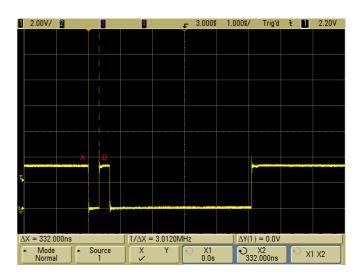
$t_{CD}$  is measured as 4420.0ns. The number of cycles calculates as follows: Cycles<sub>CD</sub> =  $t_{CD} / t_{Cycle}$ = 4420.0ns / 20.866ns = 211.83Cycles => 212Cycles
