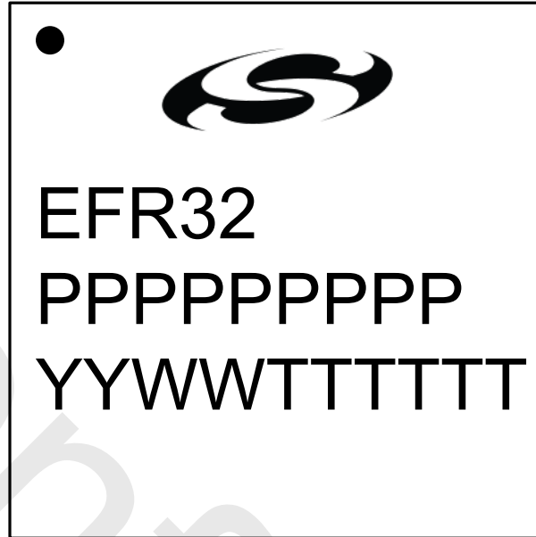
Figure 8.3. QFN32 Package Marking
