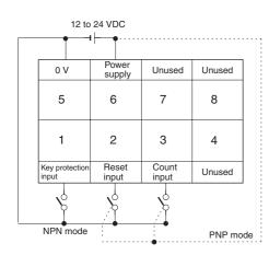
H7GP-T External power supply 12 VDC 50 mA max. 100 to 240 VAC Ń Power Powe 12 VDC 0 V supply supply 7 8 5 6 1 2 3 4 Key protection Reset Count Unused input input \ر کر NPN mode PNP mode
