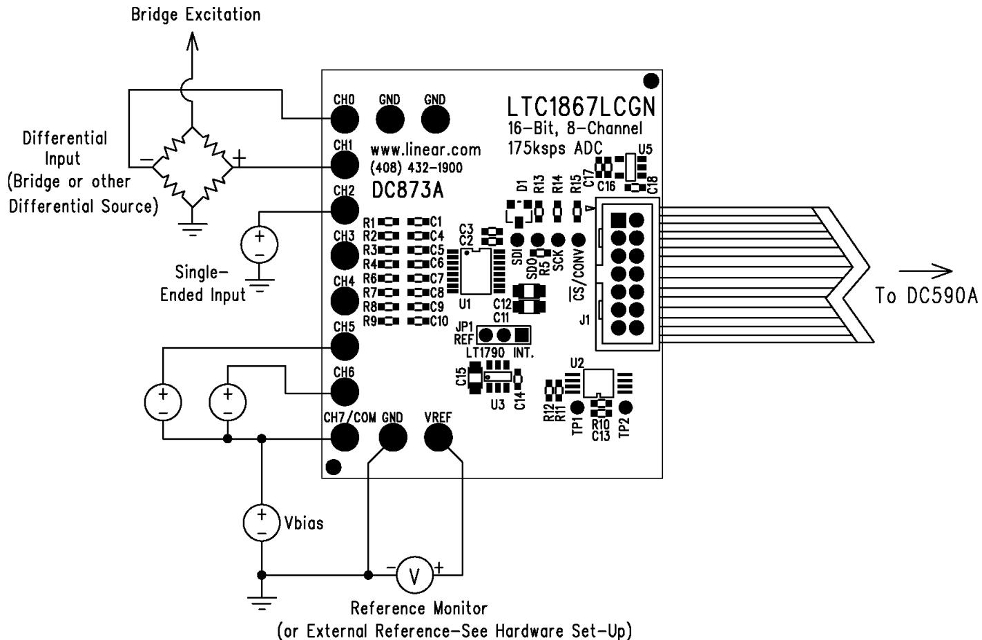
Figure 1. Connection Diagram
