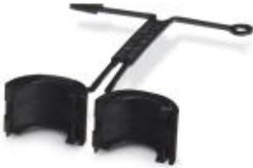
Locking clip for the pin and socket side of sensor/actuator cables with straight M12 connector and M12 connectors which can be assembled with QUICKON fast connection technology, serves to ensure M12 plug-in connections in areas with a danger of dust explosions in zone 22, according to EN 50281-1-1
