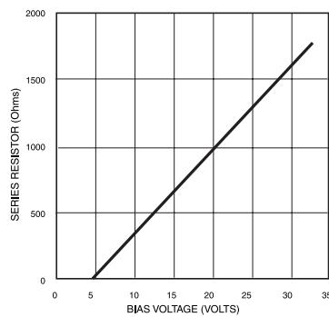
**SERIES LIMIT BIAS RESISTOR VS BIAS VOLTAGE**
