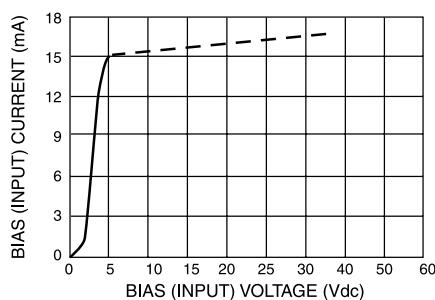
**BIAS (INPUT) CURRENT VS BIAS (OUTPUT) VOLTAGE**
