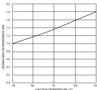
**NORMALIZED ON RESISTANCE VS JUNCTION TEMPERATURE**
