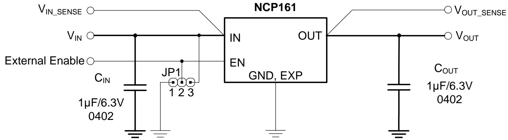
The NCP161 is 450mA high performance LDO with low quiescent current (23 $\mu$ A max.) and very high PSRR. The NCP161 also offers excellent load/line transients and ultra-low noise.
