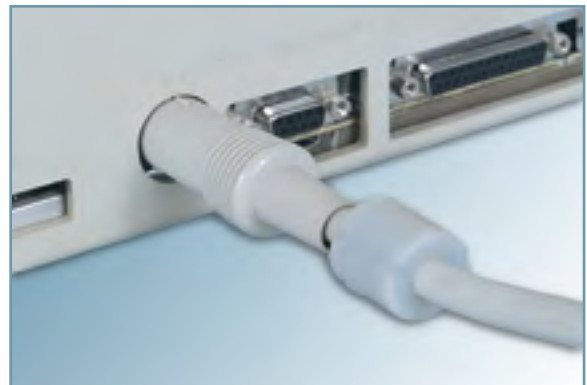
I/O cable with RFI suppressor.
