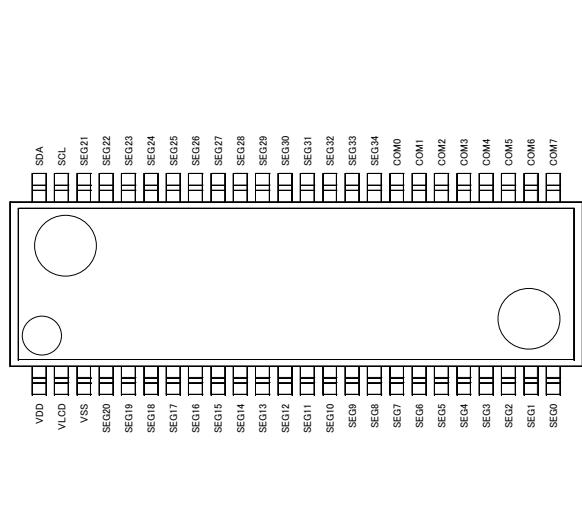
Fig.13 Pin Arrangement (BU97950FUV)
