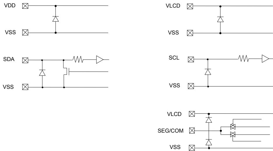
Fig.16 I/O equivalent circuit (BU97950FUV)
