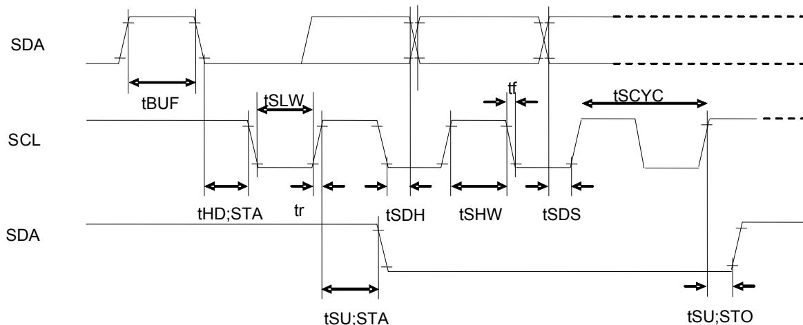
Fig.3 interface timing (BU97950FUV)
