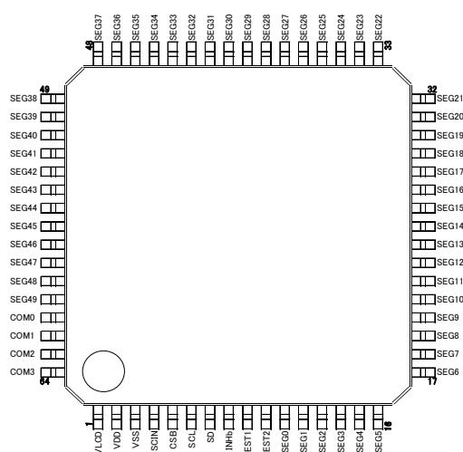
Fig.11 Pin Arrangement (BU9794AKV)
