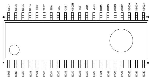
Fig.7 Pin Arrangement (BU9795AFV)
