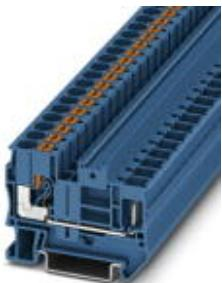
Feed-through terminal block, Connection method: Push-in / plug connection, Cross section: 0.5 mm<sup>2</sup> - 10 mm<sup>2</sup>, AWG: 20 - 8, Width: 8.2 mm, Color: blue, Mounting type: NS 35/7,5, NS 35/15
