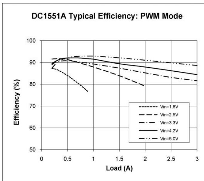
Figure 1. Typical Efficiency
