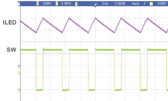
13. Steady State Waveforms
