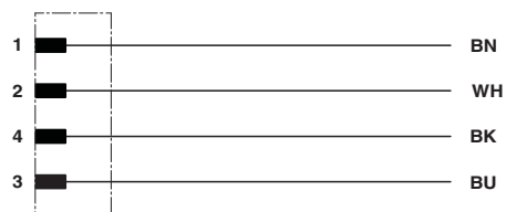
Contact assignment of the M8 plug
