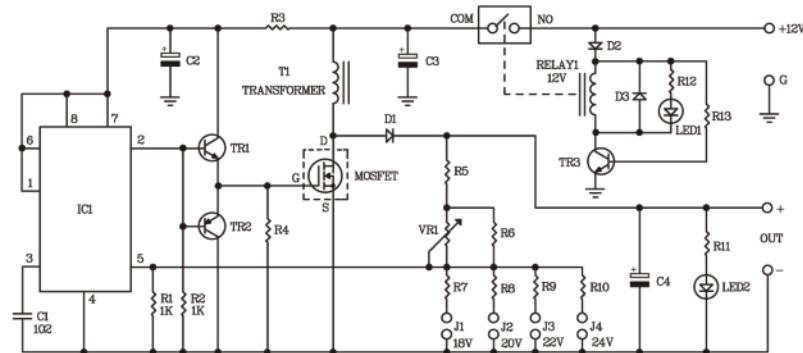
Figure 1 Voltage Booster 12 V to 15-24 V Circuit
