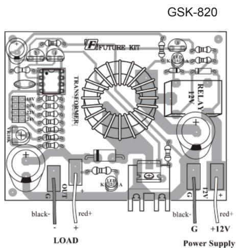
**Figure 3 Installing components**
