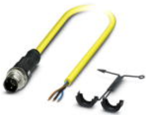
Sensor/Actuator cable, 3-position, PVC, yellow RAL 1021, Plug straight M12 SPEEDCON, A-coded, on free cable end, Cable length: 10 m
