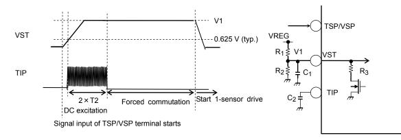
VST voltage is calculated from the following formula. (t = 0 s in startup) VST(t) = V1×(1-e^(-t/\tau)) V1 = R<sub>2</sub>/(R<sub>1</sub>+R<sub>2</sub>)×VREG (VREG = 5 V(typ.))  $\tau = (R_1 \times R_2)/(R_1+R_2) \times C_1$
