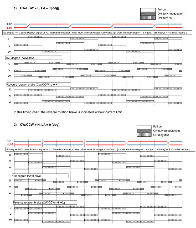
In this timing chart, the reverse rotation brake is indicated without current limit.
