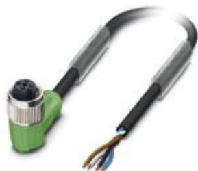
Sensor/actuator cable, 4-position, PUR halogen-free, black-gray RAL 7021, free cable end, on Socket angled M12, A-coded, cable length: 45 m
