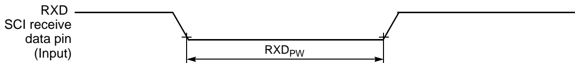
Figure 10-17 RXD Pulse Width
