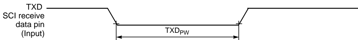
Figure 10-18 TXD Pulse Width
