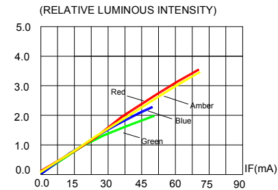
FIG.2 RELATIVE LUMINOUS INTENSITY VS. FORWARD CURRENT
