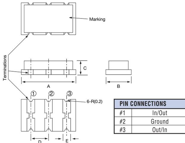
Figure 1) ECS-SR-B Series - Top, Side, Bottom & End views
