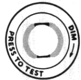
Shutters closed Minimum indirect "halo" light
