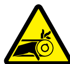
W3154 Belt Drive Entanglement Hazard
