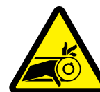
W3154 Belt Drive Entanglement Hazard
