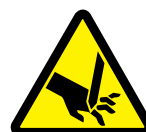
W3158 Cut or Sever Hazard
