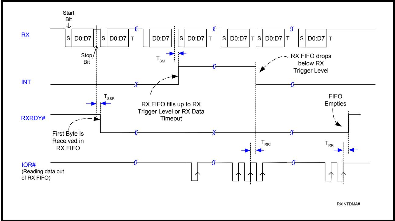
FIGURE 19. RECEIVE READY & INTERRUPT TIMING [FIFO MODE, DMA ENABLED] - PARALLEL MODE
