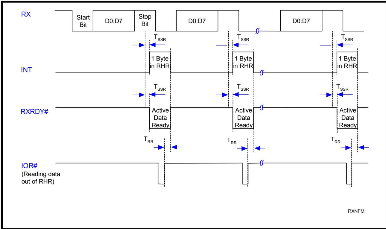
FIGURE 17. TRANSMIT READY & INTERRUPT TIMING [NON-FIFO MODE] - PARALLEL MODE
