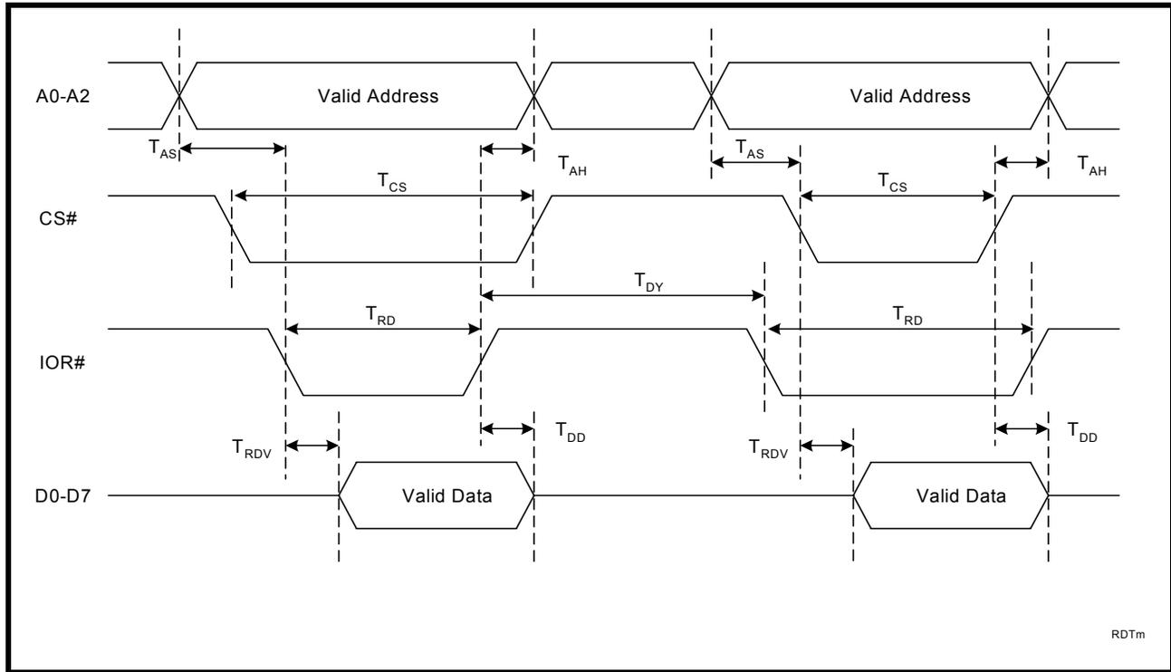
**FIGURE 13. 16 MODE (INTEL) DATA BUS WRITE TIMING - PARALLEL MODE**
