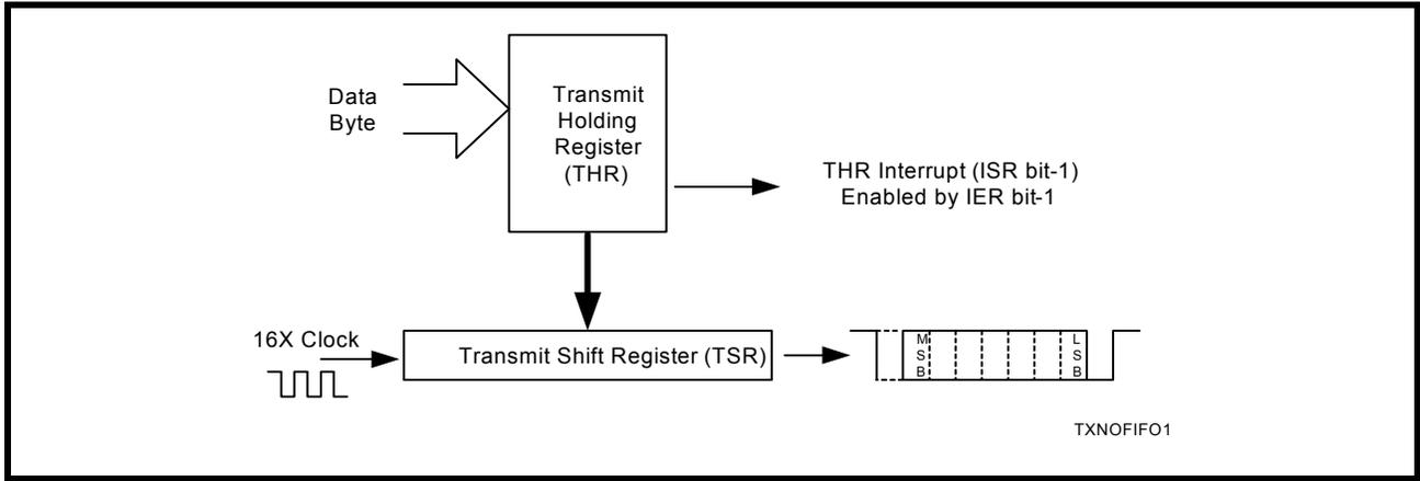
**3.9.3 Transmitter Operation in FIFO Mode**
