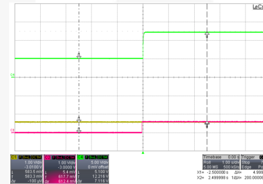
Figure 65. CH1[DP], CH2[DN], CH4[V O ] Mode Change from 5 V to 12 V
