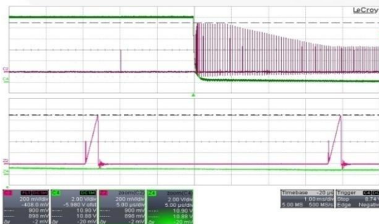
Figure 29. C2[V Cs ], C4[V O ], 264 V AC /50 Hz, I O =0 A, V O =12 V
