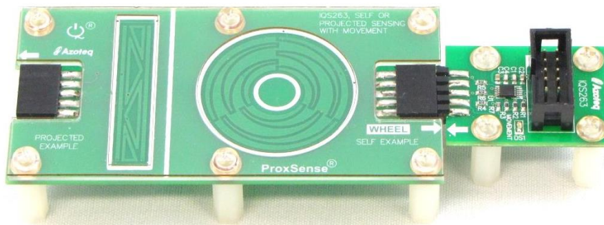
Figure 4.1 Wheel demo board connected to driver board
