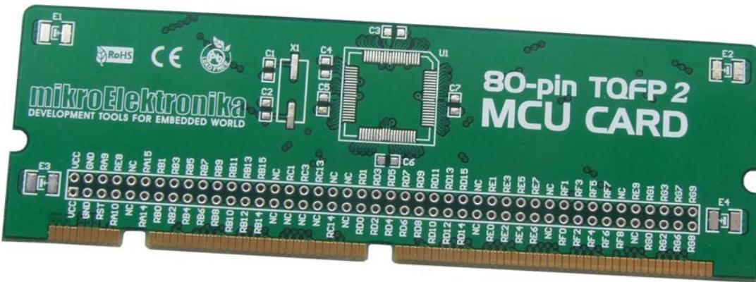
Figure 7: Empty 80-pin MCU card (TQFP2)
