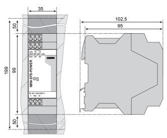
Installation: Installation depth 95 mm (+ DIN rail)
