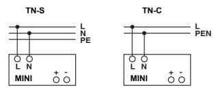
The 100...240 V AC connection is made using the L and N screw connections.
