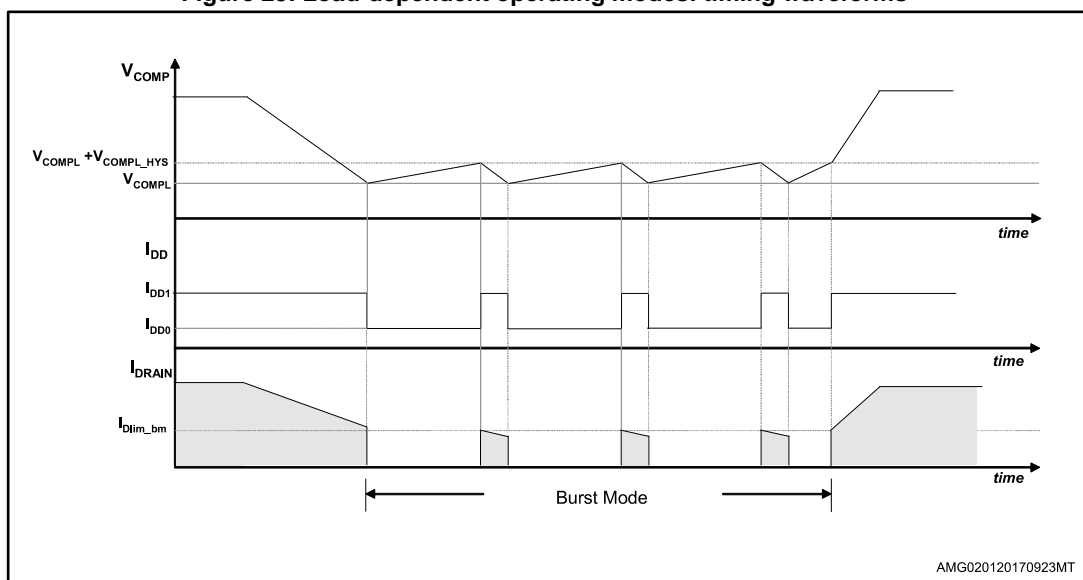
Figure 25: Load-dependent operating modes: timing waveforms
